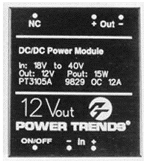
Figure 2. An example of the variety of information that can be marked on a semiconductor package.
