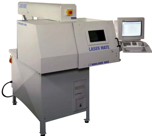
The Laser Mate II operates with high speed galvanometers.
