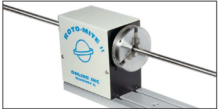
Roto-Mite rotary attachments allow marking around the diameter of cylindrical parts. They can also be used as indexers for marking on multi-sided hex or square parts.
