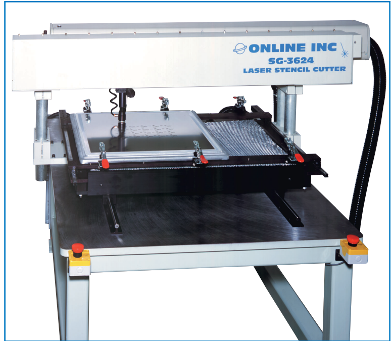
Optional hold down fixture shown in operation cutting a 24" x 24" PCB stencil.
